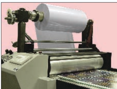
Embossing Roller (option) Swing Out Mandrel
