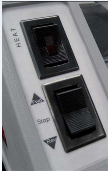
Heat & Speed Switches
