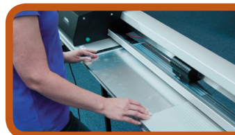
Cuts up to 3mm flexible substrates
